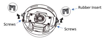
• Slightly loosen the 4 screws on the sides of the canopy, allowing the SkyPlug ample room to engage into the slot.
